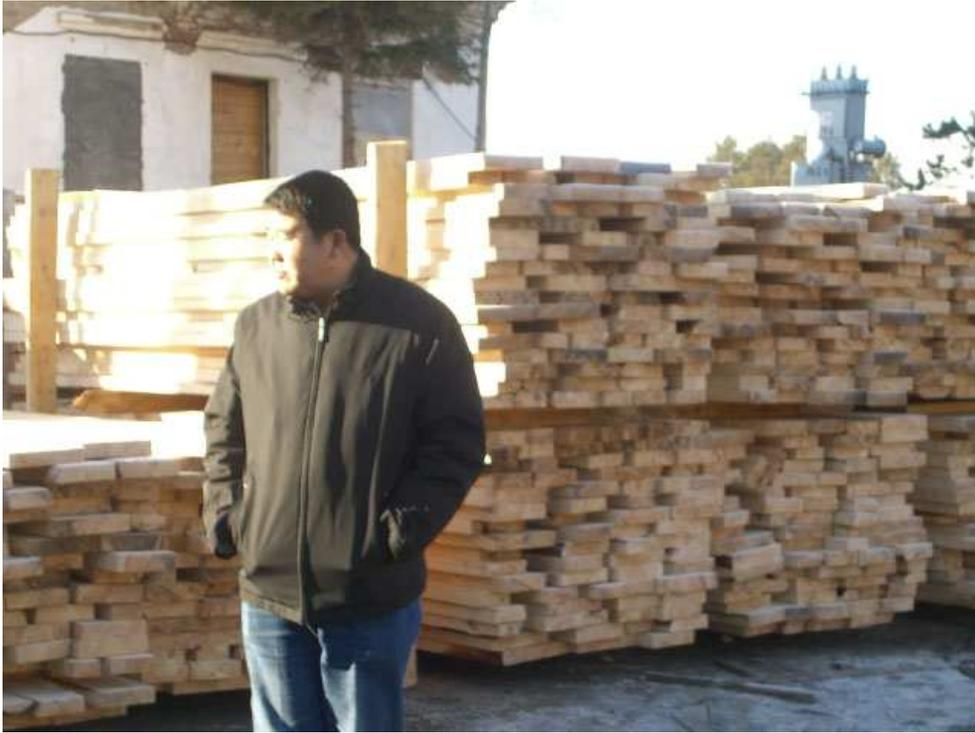
FIGURE 4.4 PINE ROUGH SAWN TIMBER STACKED AND READY FOR TRANSPORT TO RAIL DEPOT
